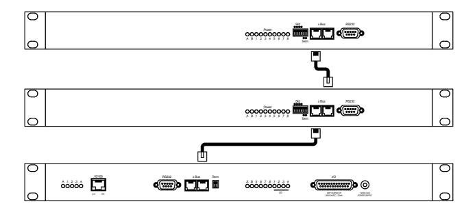
2. Allocate an address to each Satellite by positioning the address selection DIP-switches marked "Slct" on the front panel according to the following table.
