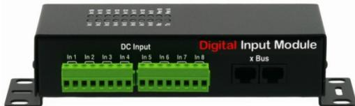
Up to 16 Digital Input Modules with 16 inputs for dry contacts (door contacts, smoke and water detectors...) can be attached to the ePowerSwitch 8XM to monitor environmental conditions.
