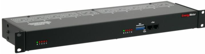
Up to 16 EnergyMeters can be attached to the ePowerSwitch 8XM to monitor the energy consumption (kWh) and the current consumption (Amp RMS) of eight electrical devices (PC, server, light, printer...) and trigger actions if predefined limits are exceeded. The EnergyMeter is also able to monitor the Input voltage of both 16 Amps power inputs.
